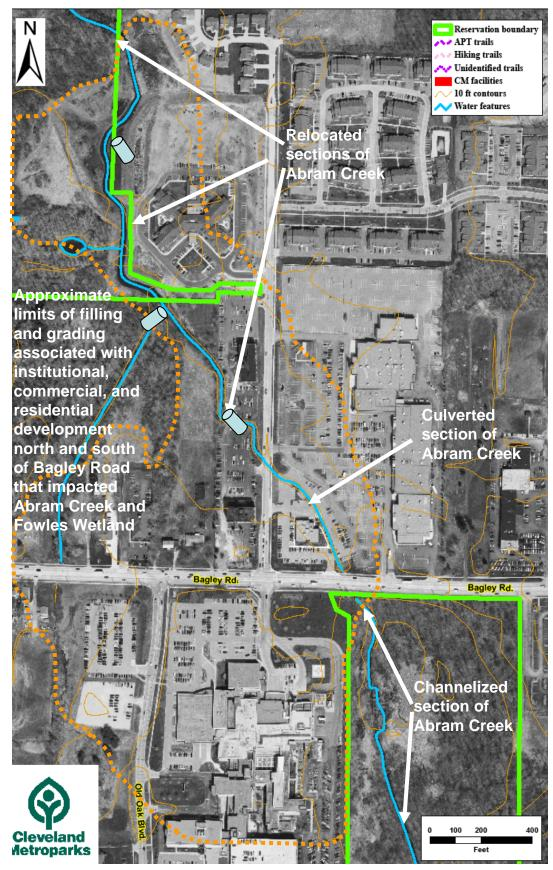
Figure 16B. Middle area of Lake Abram ecosystem showing areas of fill, channelization, culverting, and relocation of Abram Creek.
