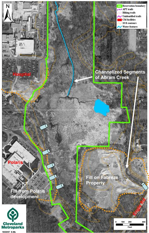
Figure 16C. Southern end of Lake Abram ecosystem showing Fowles Wetland area and areas of fill, stream channelization, development, and known stormwater inputs. = known or suspected storm water input location.
