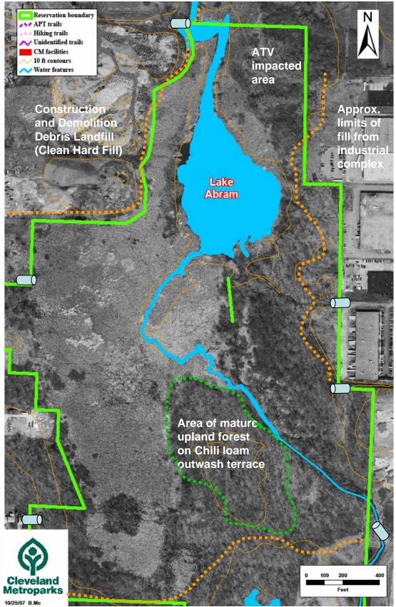
Figure 16A. Upper area of Lake Abram ecosystem showing areas of fill, channelization, and storm water inputs. = known or suspected storm water input location.
