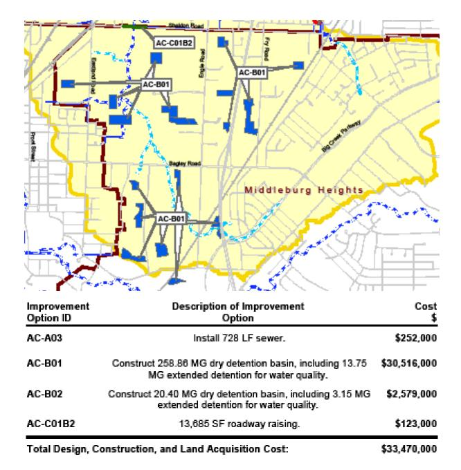
Figure 18. Storm water detention facilities recommended in the RIDE Study for Abram Creek watershed (NEORSD 2004).
