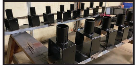
Boardwalk sill caps and other brackets are welded, cleaned, and painted in-house with Site Construction's support.
