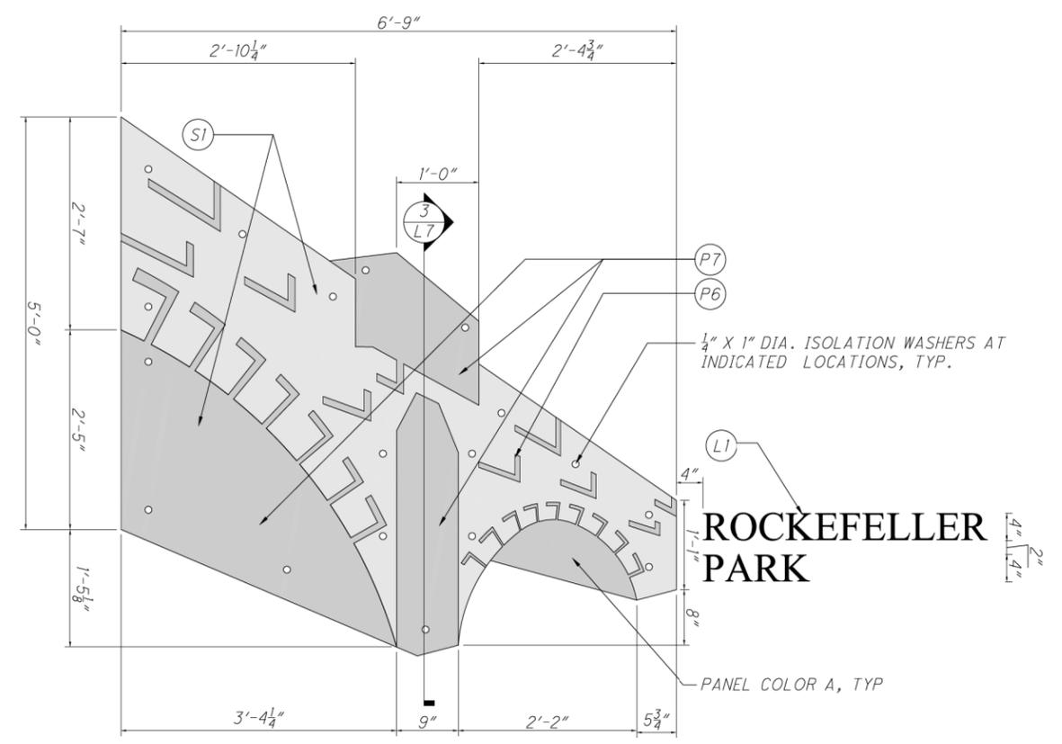
NOTE: SIGN COMPONENT TO FOLLOW RADIUS OF ABUTMENT WALL. IF RADIUS CANNOT BE ACHIEVED, VERIFY SPACERS, AS NECESSARY TO COMPENSATE FOR CURVED WALL. VERIFY WITH ARCHITECT (PROVIDE MOCK-UP) PRIOR TO FABRICATION / INSTALLATION, TYP. SIGN CAD FILE IS AVAILABLE TO CONTRACTOR FOR FABRICATION.
