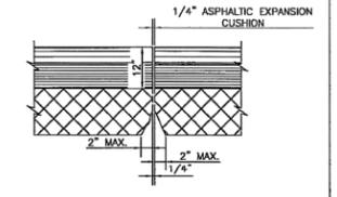
ELEVATION SHOWING CURB JOINT SECTION "A" - "A"
