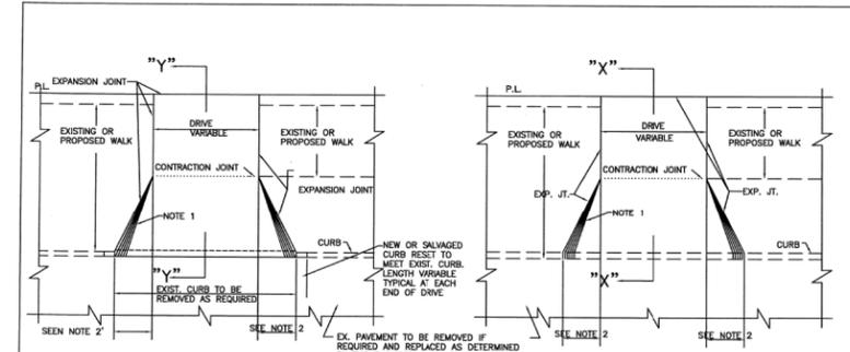
PLAN FOR NEW DRIVE WITH INTEGRAL CONCRETE CURB
