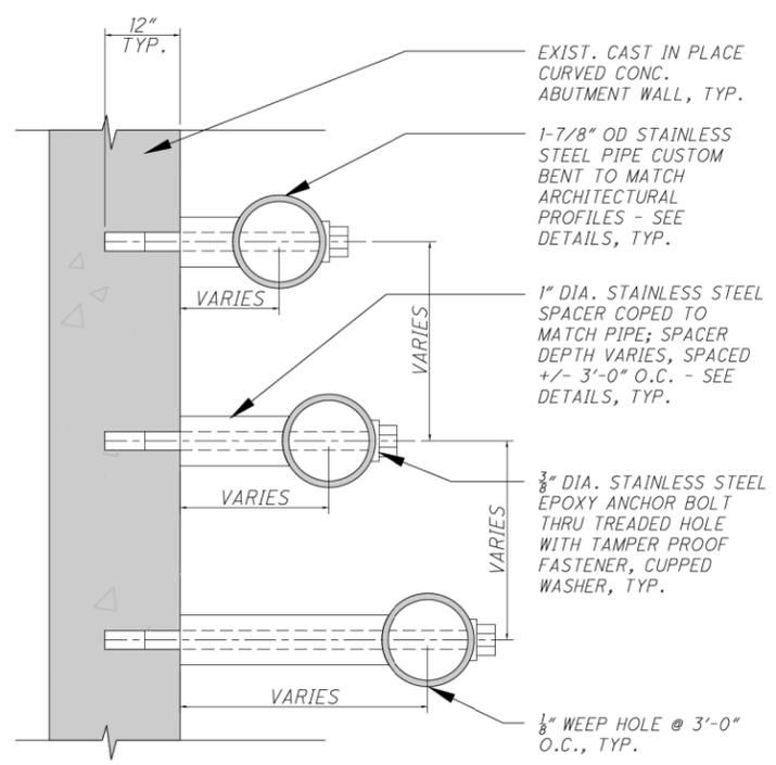
EXIST. CAST IN PLACE CURVED CONC. ABUTMENT WALL, TYP.
