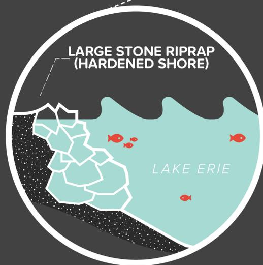
+ Larger stone revetments protect the Isle from high lake levels and intense wave action, allowing for the creation of a protected and natural cove.
