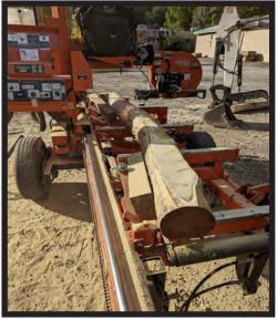
We mill just the top of these logs to make natural timber steps.
