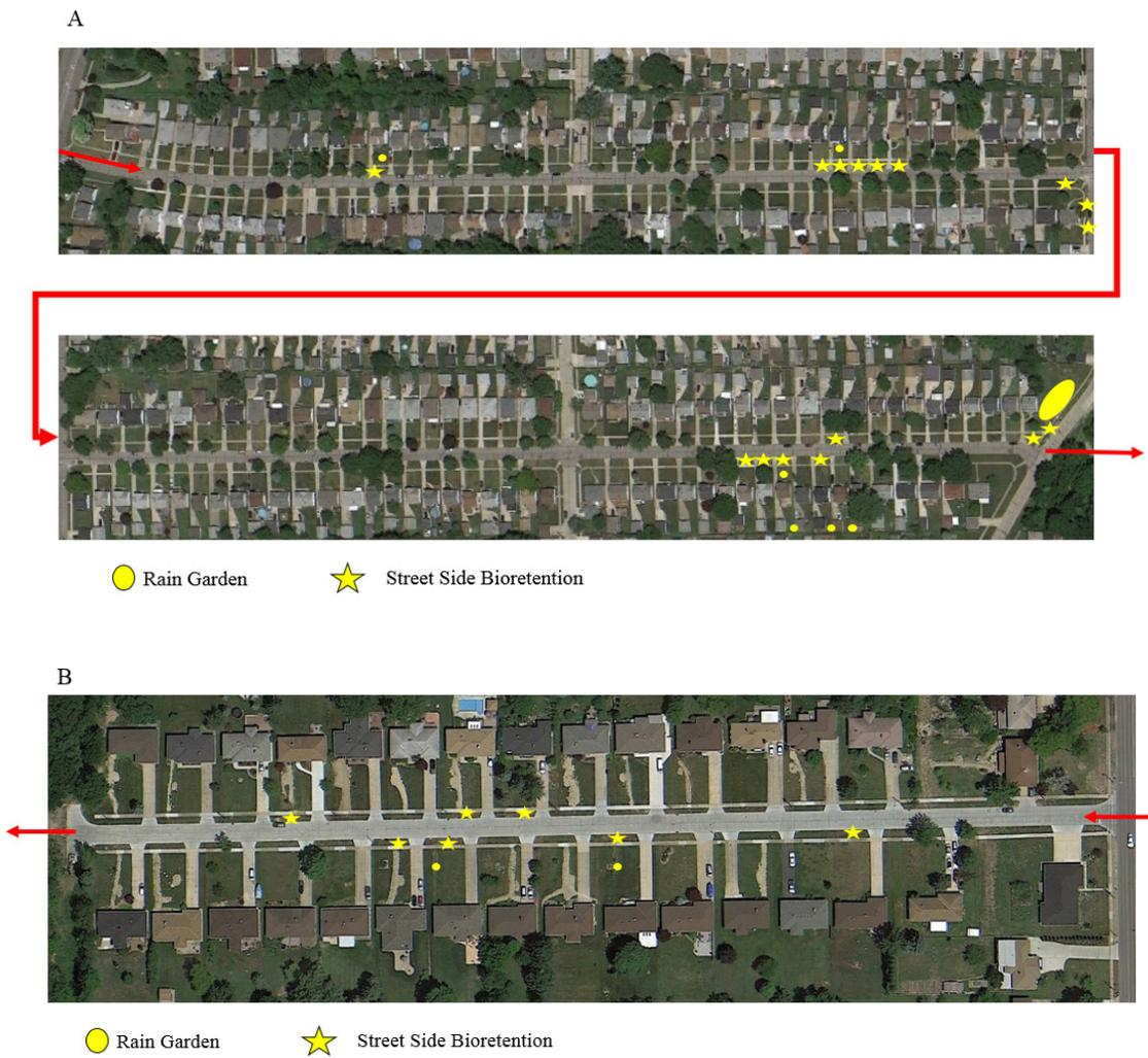
Figure 1-3. Overview map showing locations for rain gardens and street side bioretention gardens on (A) Klusner and (B) Parkhaven (Red arrows indicate the general direction of stormwater flow on each street).
