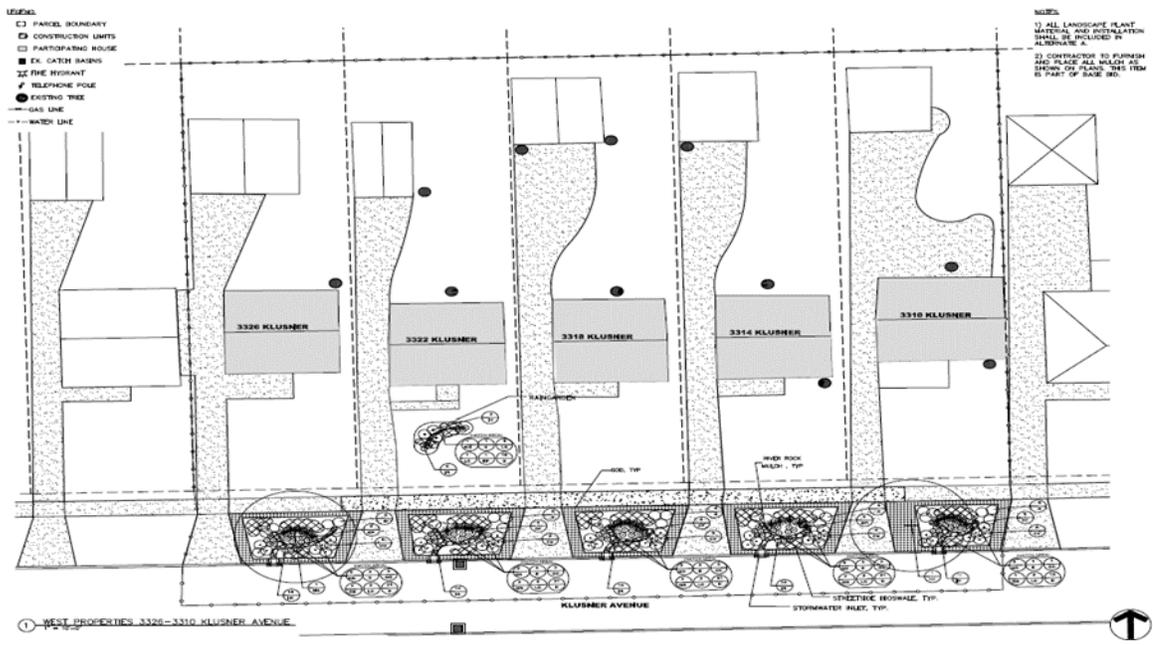
Figure 1-4. Typical site design for street side bioretention gardens and rain gardens at West Creek Watershed Parma, Ohio. Black dots represent the locations of rain barrels. (URS Design, 2013).
