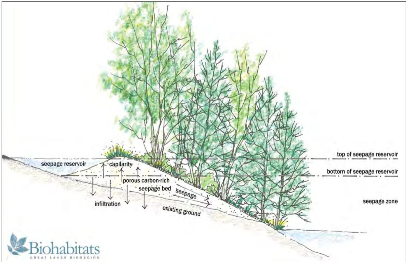
Figure 40. A typical cross section of a sand seepage berm design (Copyright Biohabitats Inc.).
