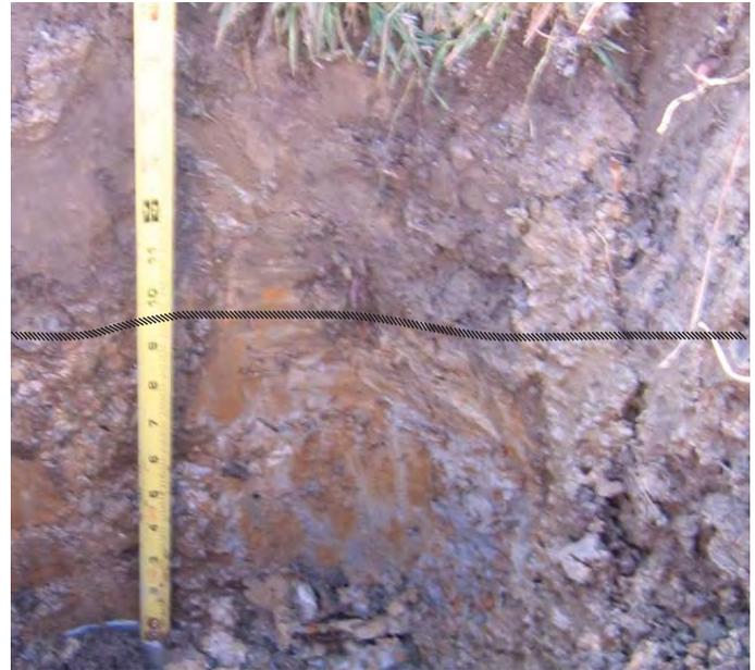
Figure 10. Discontinuity between surface and subsurface soil layers. Line on photo shows approximate location of change in texture.
