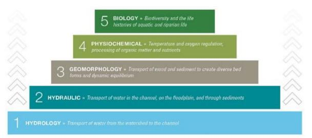
Figure 12. The functional pyramid sets a hierarchy of values to ensure that key processes are not overlooked during the design process for stream restorations. It is structured according to the modifications that are necessary to ensure functionality. For example, physicochemical traits such as temperature (4) cannot be restored without the appropriate geomorphology (3) (source: StreamMechanics, Harman et. al., 2012).
