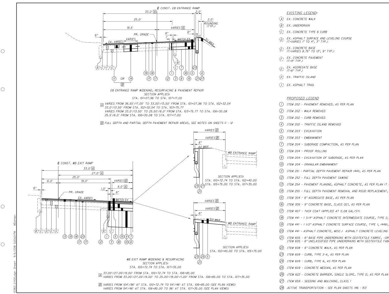
S Ζ TIO C ш S ∢ C ٩ > (13) ITEM 254 - PAVEMENT PLANING, ASPHALT CONCRETE, AS PER PLAN (T = VARIES) (14) ITEM 255 - FULL DEPTH PAVEMENT REMOVAL AND RIGID REPLACEMENT, CLASS QCI, AS PER PLAN (18) ITEM 441 - 1 3/4" ASPHALT CONCRETE INTERMEDIATE COURSE, TYPE 2, (448) (19) ITEM 441 - 1 1/2" ASPHALT CONCRETE SURFACE COURSE, TYPE 1, (448), PG70-22M, AS PER PLAN 02  $\langle \! O \!
