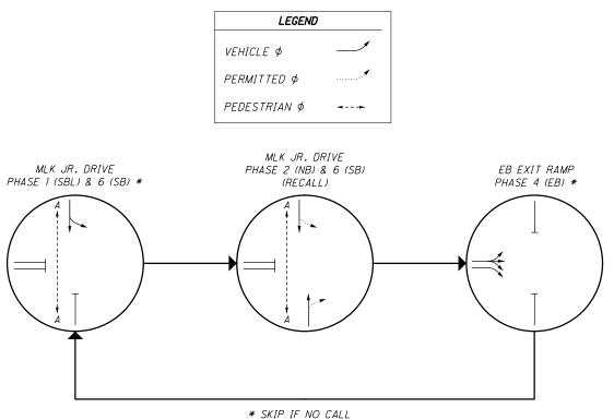
\*VOLUME DENSITY CONTROLS COUNTDOWN PEDESTRAIN SIGNALS SHALL GO TO ZERO ON YELLOW PER OMUTCD FIGURE 4E-2 PEDESTRIAN PHASE TO REST IN WALK
