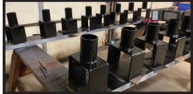
Boardwalk sill caps and other brackets are welded, cleaned, and painted in-house with Site Construction's support.
