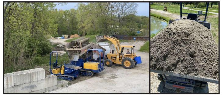
All of our trail stone is sourced locally from facilities that mine native bedrock that matches the geology of the park district. The mineral content is the perfect mix for bonding and drainage. Unlike limestone, it will not affect the pH of the surrounding soil. Our trail surface material is then screened in-house to create a finer material that improves compaction and stays in place and is durable under all weather conditions.
