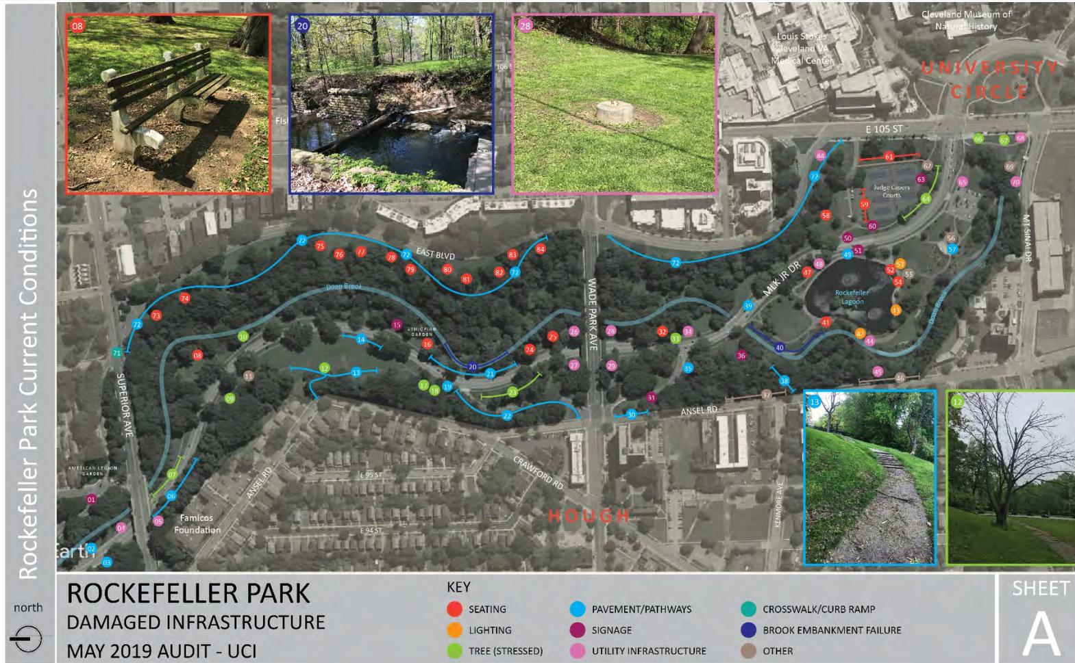
Figure 11. Rockefeller Damaged Infrastructure Audit, Source: University Circle Incorporated
