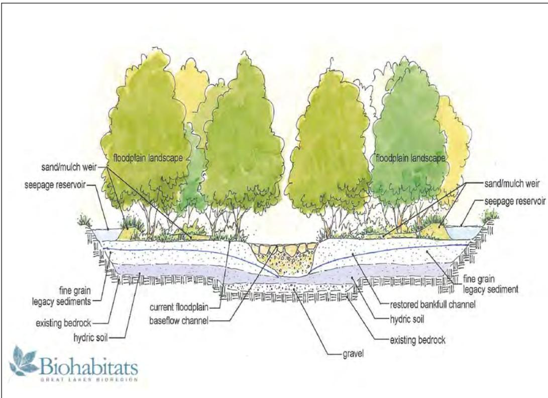
Figure 36. A typical cross section of floodplain reconnection (Copyright Biohabitats Inc.).
