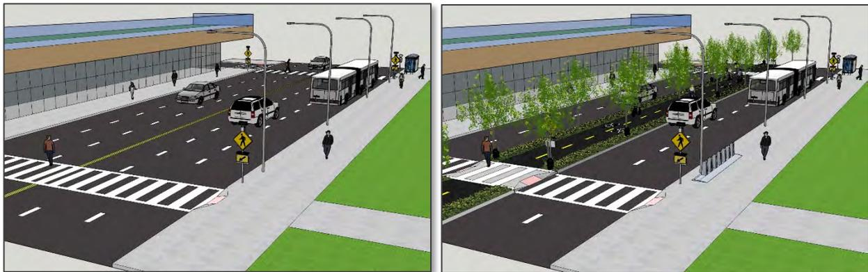
*Figure 8. 'Before' and 'After' Views of a Midway Cycle Track Corridor*
