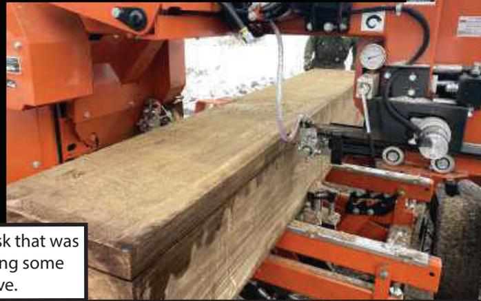
The new Woodmizer bandsaw mill is able to rotate logs through hydraulics, a task that was previously done by hand. An on-board computer sets the cutting depth creating some of the most consistent boards we have seen since we started the initiative.
