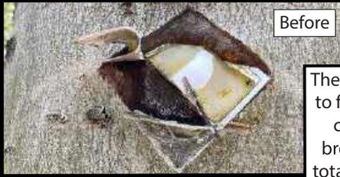
The old markers were set up to fail after just a few years, causing signs to either break off or end up being totally engulfed by the tree.
