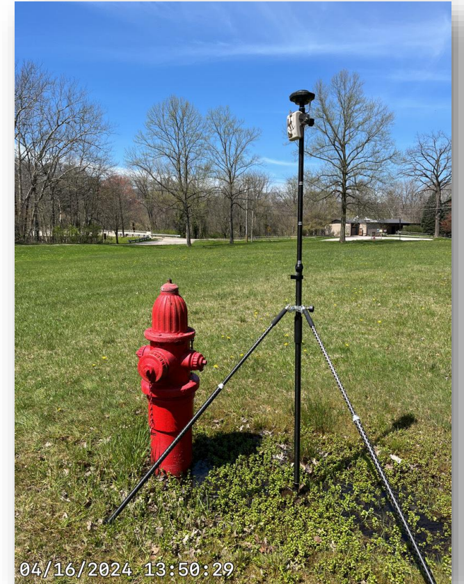
Rocky River Reservation, Stables – GPS collection of hydrants, April 2024
